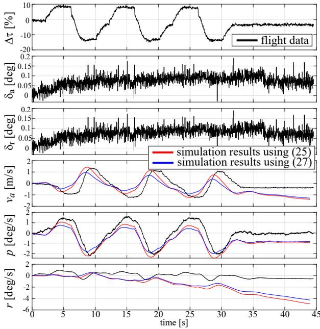
Fig. 4. Flight data #1 for asymmetric torque input (black lines), and simulation results with estimated  $B(\hat{\theta})$  in (25) (red lines) and estimated  $B(\hat{\theta})$  in (27) (blue lines)
