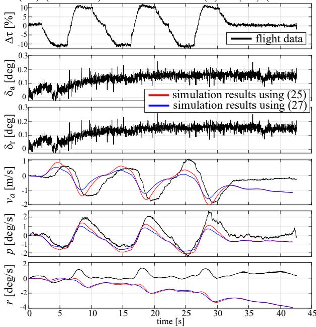
Fig. 5. Flight data #2 for asymmetric torque input (black lines), and simulation results with estimated  $B(\hat{\theta})$  in (25) (red lines) and estimated  $B(\hat{\theta})$  in (27) (blue lines)
