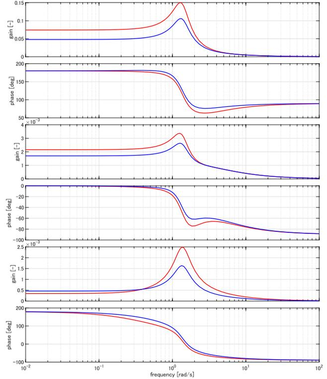
Fig. 6. Bode plots of  $G(z, \hat{\theta})$  using  $B(\hat{\theta})$  in (25) (red lines) and  $B(\hat{\theta})$  in (27) (blue lines)
