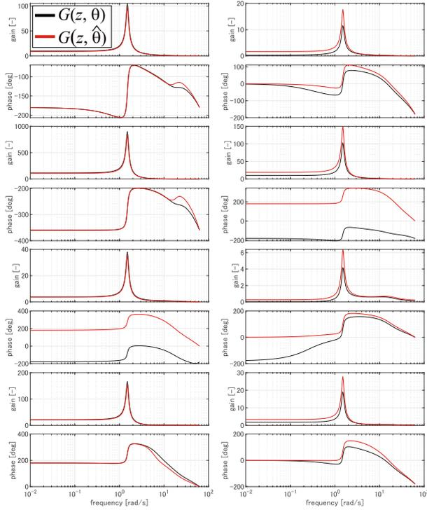
Fig. 2. Bode plots of  $G(z, \theta)$  with actual  $B$  (black lines) and  $G(z, \hat{\theta})$  with the estimated  $B(\hat{\theta})$  in (21) (red lines)
