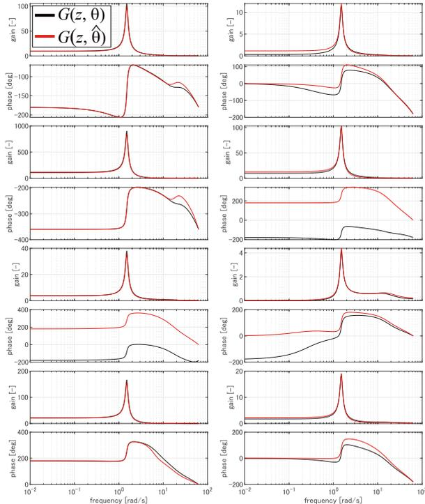
Fig. 3. Bode plots of  $G(z, \theta)$  with actual  $B$  (black lines) and  $G(z, \hat{\theta})$  with the estimated  $B(\hat{\theta})$  in (23) (red lines)
