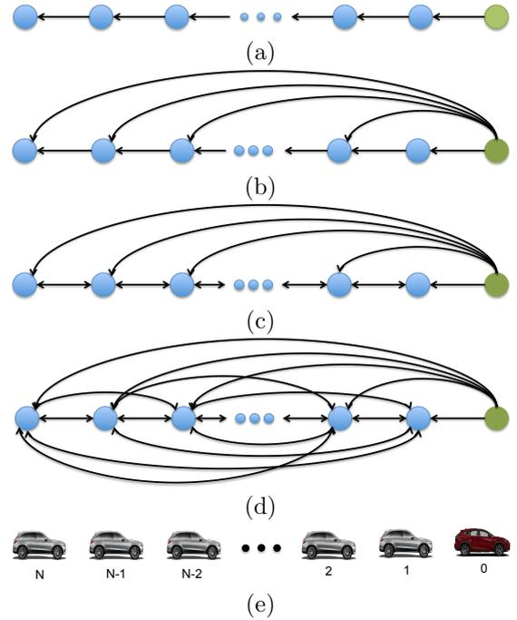
Fig. 1. Exemplar platoon communication topologies (Fiengo et al., 2019): (a) Predecessor-Following (P-F), (b): Leader-Predecessor-Following (L-P-F); (c): Bidirectional-Leader (B-D-L); (d): All-to-All (Broadcast, BR); (e): Platoon of  $N$  vehicles plus a leader.
