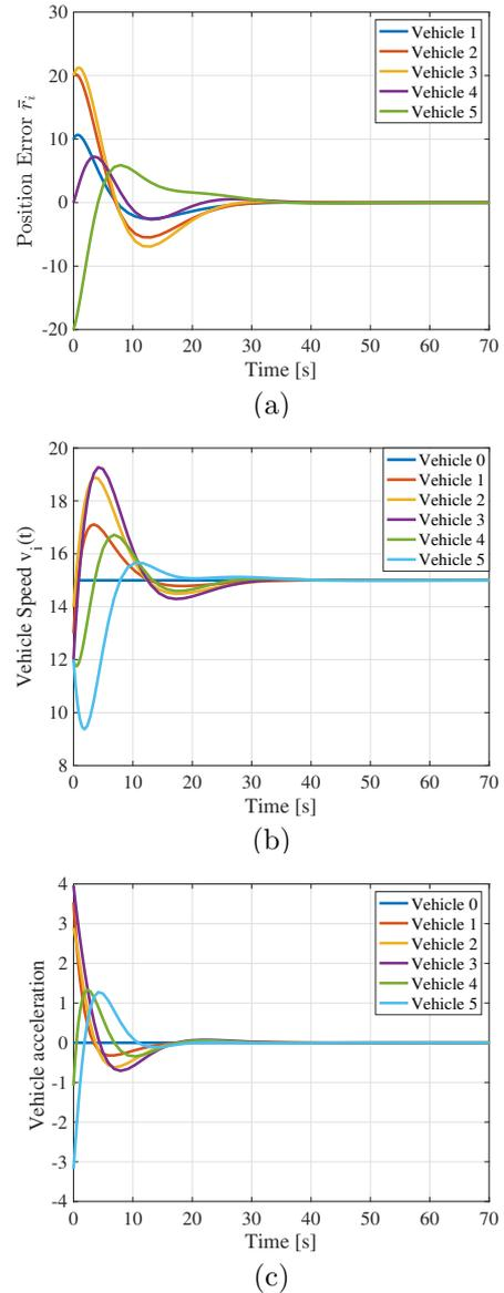
Fig. 2. Leader tracking performance under the distributed PI control in (6). Time history of: a) inter-vehicle distances  $p_i(t) - p_0(t) - d_{i0}$  ( $i = 1, 2, 3, 4, 5$ ); b) vehicles speed  $v_i(t)$  ( $i = 0, 1, 2, 3, 4, 5$ ); c) vehicles acceleration  $a_i(t)$  ( $i = 0, 1, 2, 3, 4, 5$ ).
