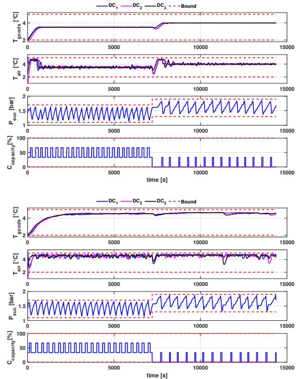
Fig. 2. Tracking (upper) and economic (lower) results of using the Bi-level nonlinear MPC approach
