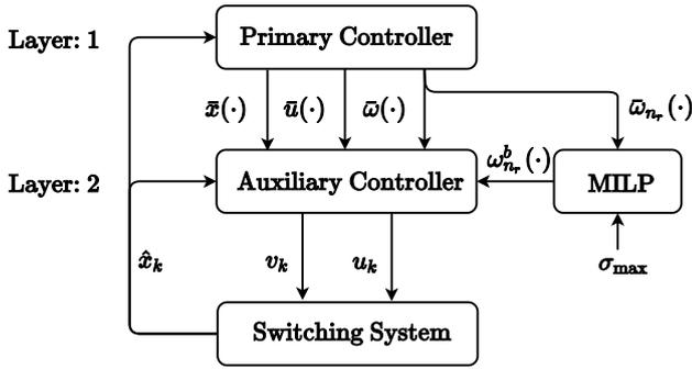
Fig. 1. MPC scheme for switching systems
