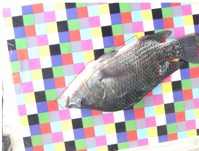
Fig. 9. Image characteristics that have confused the stereo match algorithm to create the disparity map (sunlight reflection on the fish and monochrome areas)
