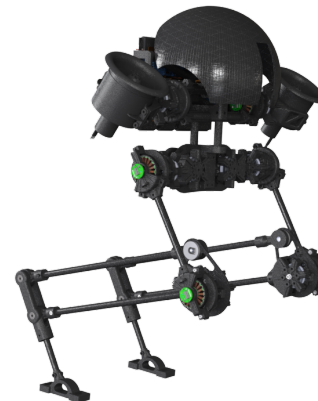
Fig. 1. CAD model for a thruster-assisted bipedal robot designed by the authors
