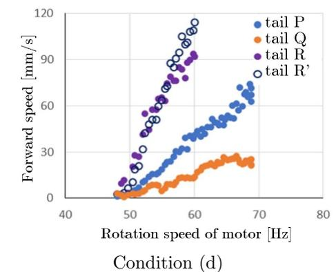
Fig. 7. Experimental results of forward swimming speed
