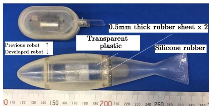
Fig. 1. Miniature aquatic robots utilizing resonance of elastic plate (upper) and body (lower)
