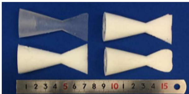
Fig. 4. Casted elastic tails: P (Left up), Q (Left down), R (Right up) and R' (Right down)
