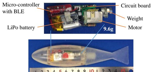
Fig. 3. Micro-controller and vibration motor inside robot
