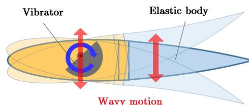
Fig. 2. Principle of propulsion
