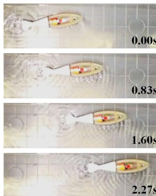
Fig. 6. Example of forward swimming of robot
