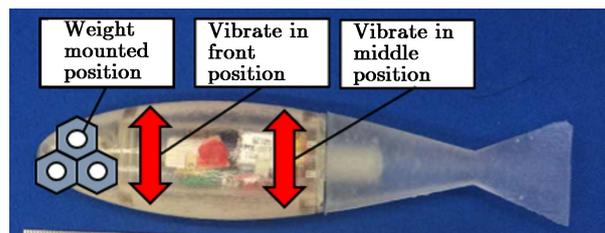
Fig. 5. Position of weight and vibrator
