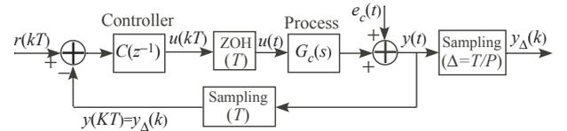
Fig. 3. Process model in closed-loop system
