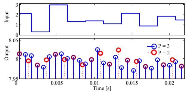
Fig. 2. Illustration of experimental input-output data. From the top: input  $u(t)$ ; Output  $y_\Delta(k)$  for  $P = 2$  (dashed) and  $P = 3$  (solid).
